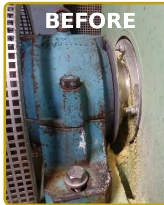
MECO AH TYPE-2S, ON A 6.69" (170mm) SHAFT ON A FILTER PRESS SEALING DAMP CORN STARCH
