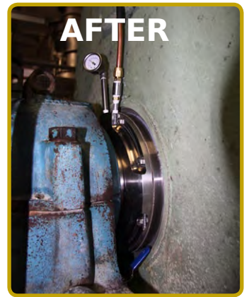
MECO AH TYPE-2S, ON A 6.69" (170mm) SHAFT ON A FILTER PRESS SEALING DAMP CORN STARCH
