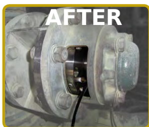
FIG. 3 MECO AH TYPE-2S ON A 3" (76MM) SHAFT ON A SCREW FEEDER CONVEYING DRY SULFUR POWDERS.
