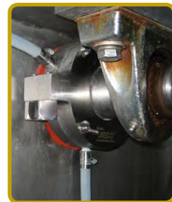
FIG. 1 MECO AH TYPE-2 DAIRY SEAL, INSTALLED ON A DAIRY CREAMER
