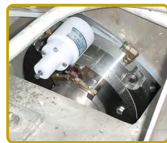
FIG. 2 MECO AH TYPE-2S FOR CERTAIN EUROPEAN EXPLOSIVE ATMOSPHERE APPLICATIONS, WHERE EN 94/9/EC COMPLIANCE IS REQUIRED.
