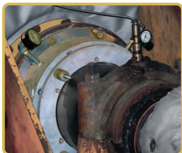
MECO EP T3 INSTALLED ON A PRESSURIZED DRYER
