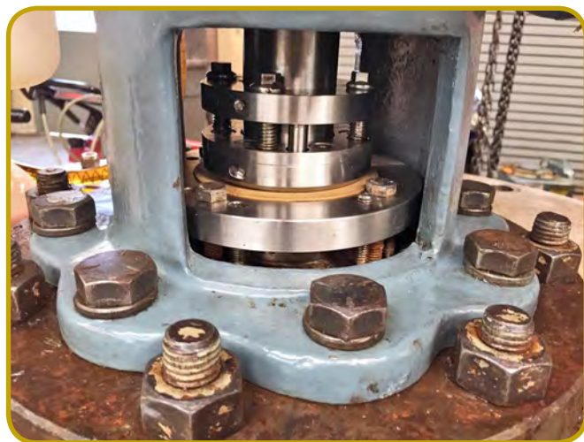
2" OFS TYPE-1 SEAL INSTALLED ON A TOP-ENTRY AGITATOR CONTAINING VOCs AND MOLTEN PLASTIC RESIN
